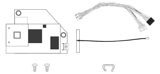
The Wireless LAN module provides Wireless LAN connectivity for your printer.
