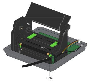
2. Plug the cutter connector to the **J8** on the main board. **J8** is a white port
