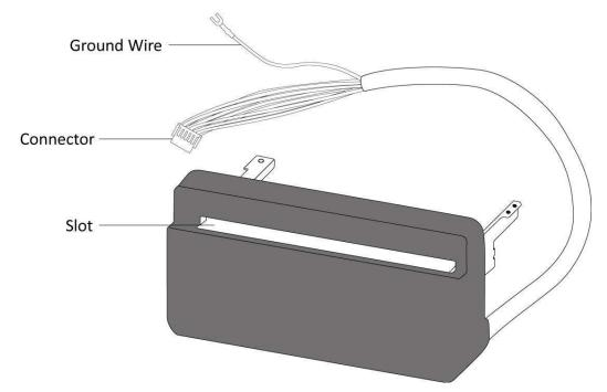
A cutter is used to cut the label after it is printed out. A full cutter cuts a label off from a media roll.
