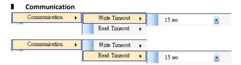
It includes **Write Timeout** and **Read Timeout**. They determine how long your computer (or other devices) waits printer's response when it attempts to write or read data to your printer. The default value is 15 seconds, meaning that the computer waits 15 seconds and displays an error message if it doesn't receive any response.
