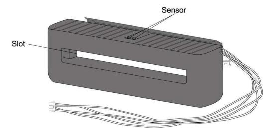
A dispenser automatically removes the liner from the printed label. The dispenser sensor detects if a peeled label is taken away.
