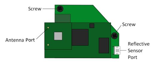
2. Below the main board, you'll find two screw holes on the lower-right. Align the two holes on the Wireless LAN card with them and secure the card with two screws.
